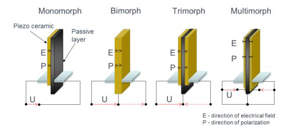
One-sided clamping is normally chosen to make use of the deflection and controlling force at the other end of the bending actuator. The ceramic layers are actuated electrically. The inverse piezoelectric effect gives rise to mechanical stress which results in a bending of the compound.
